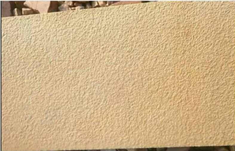
Sand Blast Finish
